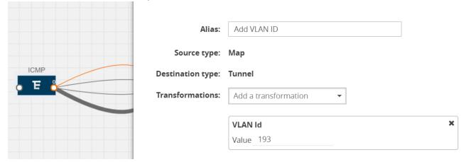
**NOTE:** Do not apply VLAN Id and VLAN PCP transformation types with the Strip VLAN ID transformation type on the same link.
